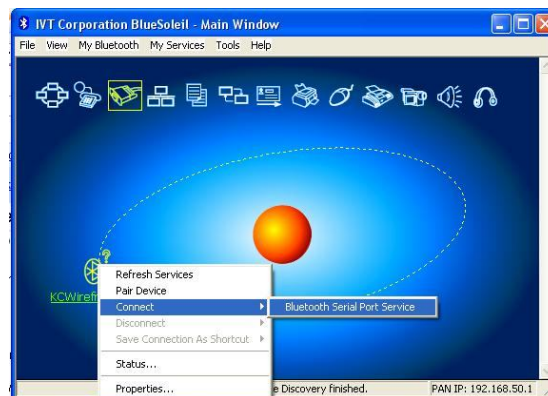
Figure 4.5: USB dongle connect to the Bluetooth Module
