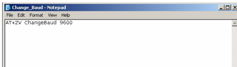
Figure 3.8: Changing baud rate command written in the Microsoft Notepad
