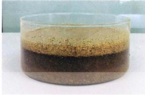
Figure 3.6 Kenaf short fibre soaked with 5% NaOH solution
