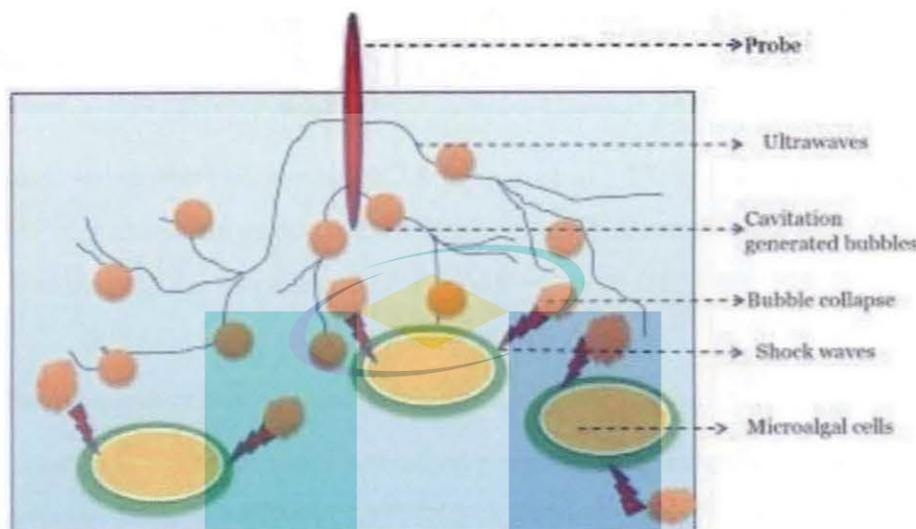
Figure 2.2 Working principle of ultrasonication for lipid extraction
