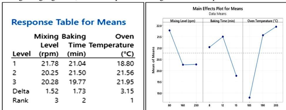
**Figure 11.** Means response table and main effects plot.
