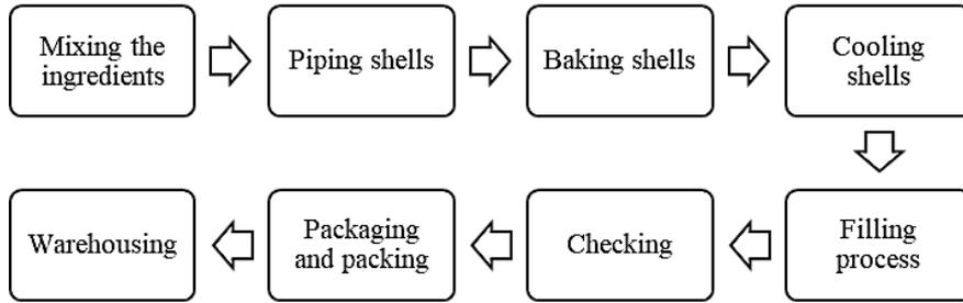
**Figure 3.** Flowchart of the current production process of macarons product.
