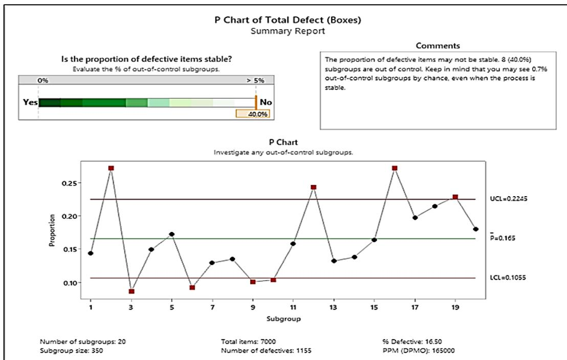
Figure 5. P-Control Chart of the total defect.
