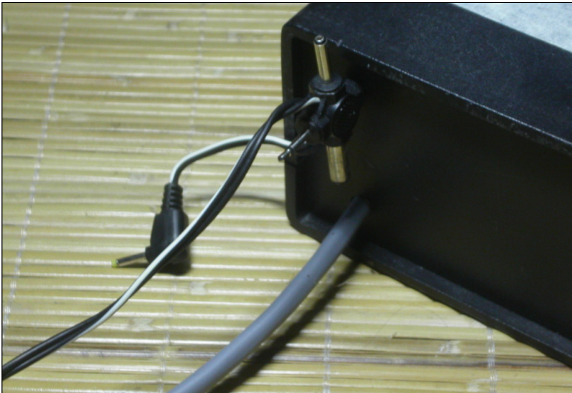
Figure 3.17 Power source for the module. 240Vac and 9Vdc for input source.
