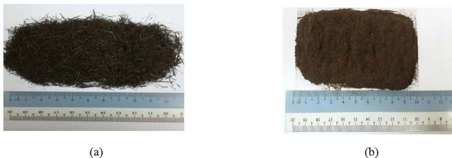
Fig. 1. (a) Arenga Pinnata fibers after cleaned and dried; (b) Arenga Pinnata powder of size 0.16 mm.
