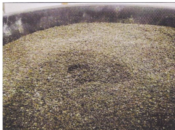
Fig. 2. Coal bottom ash.
