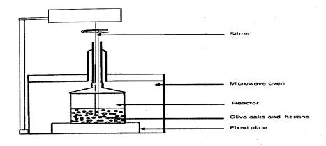
**Figure 2.1**: Schematic diagram of microwave-assisted extraction system (MASE) (*Armani and Kadi, 2010*).
