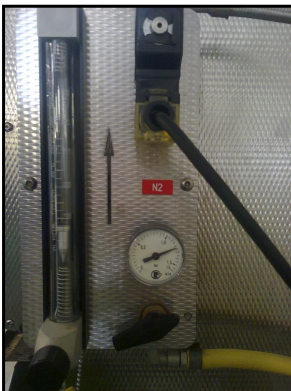
Figure 4.1: Nitrogen Gasses flow into the furnace
