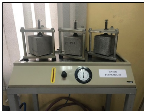
Figure 6. Water permeability test device.
