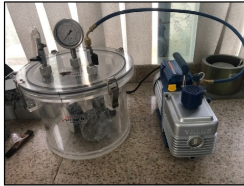
Figure 5. Water absorption test device.
