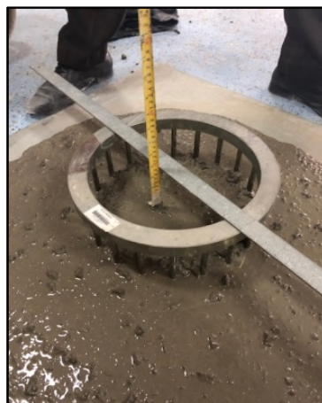
Figure 4. J-ring flow test.
