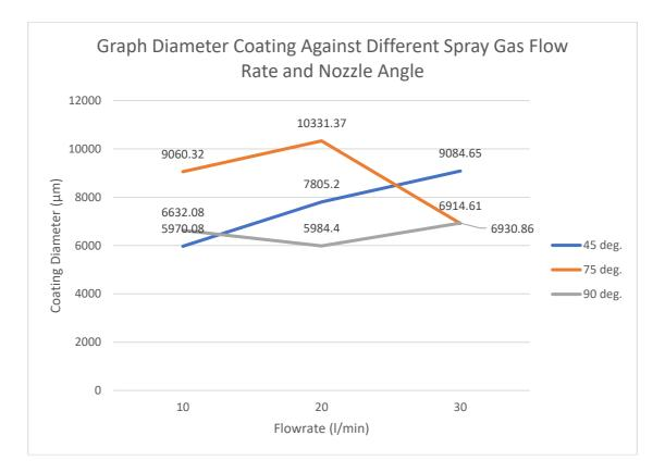
Figure 3. Coating Diameter Against Different Flow Rate Spray Gas and Nozzle Angle
