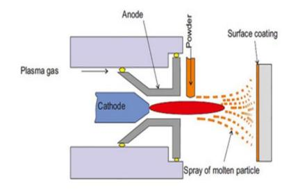
Figure1. Plasma Spraying Diagram Source:Devasia et al., 2021
