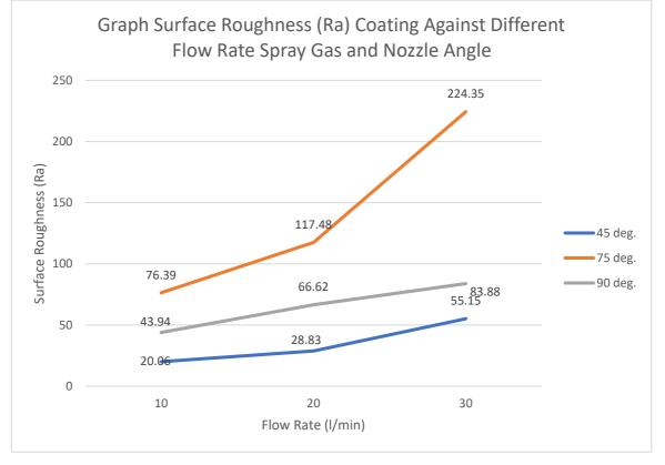
Figure 5. Coating Surface Roughness (Ra) Against Different Flow Rate Spray Gas and Nozzle Angle
