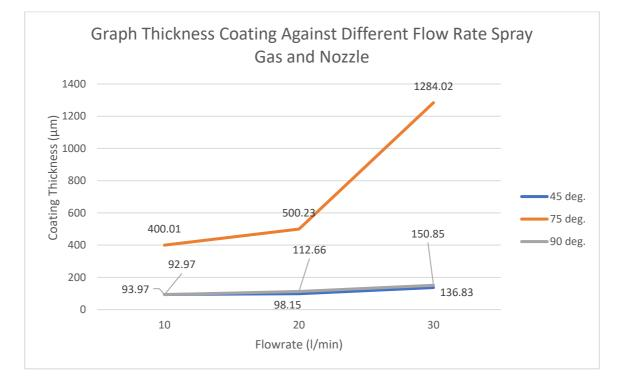
Figure 4. Coating Thickness Against Different Flow Rate Spray Gas and Nozzle
