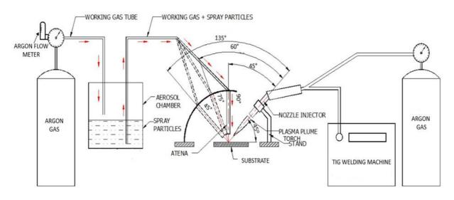
Figure 2: Schematic Representation of TIG Welding Machine with Plasma Arc Deposition
