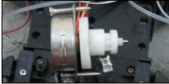
Figure 3.29: Modified stepper motor
