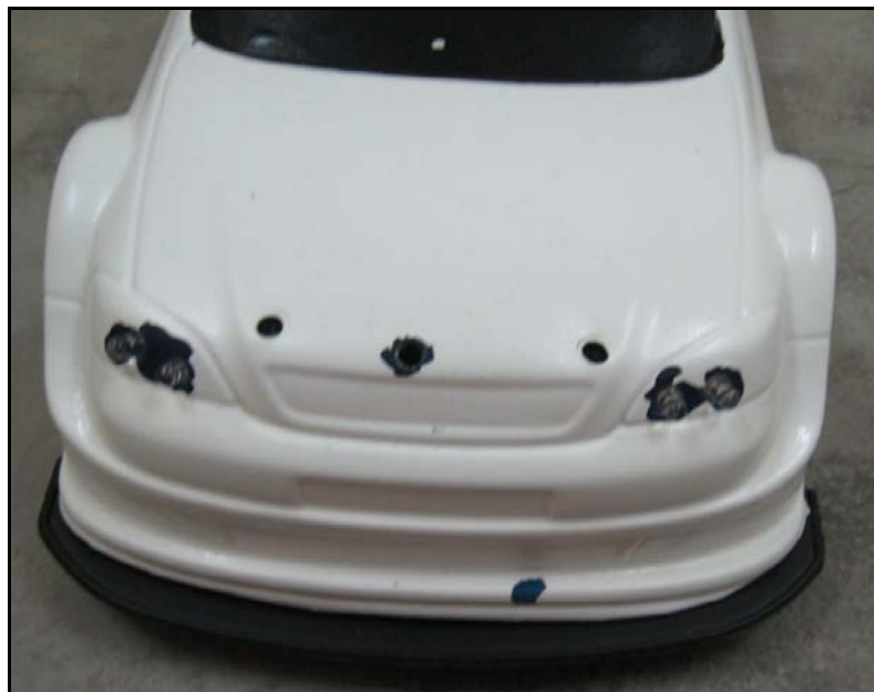
Figure 4.14: LEDs placed at the front of the car
