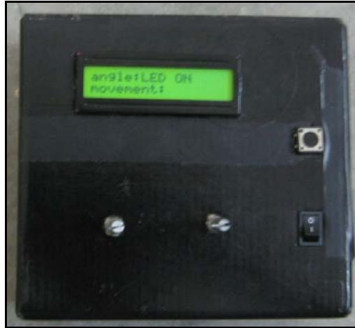
Figure 4.9: LCD is inserted into the slot at the remote control box
