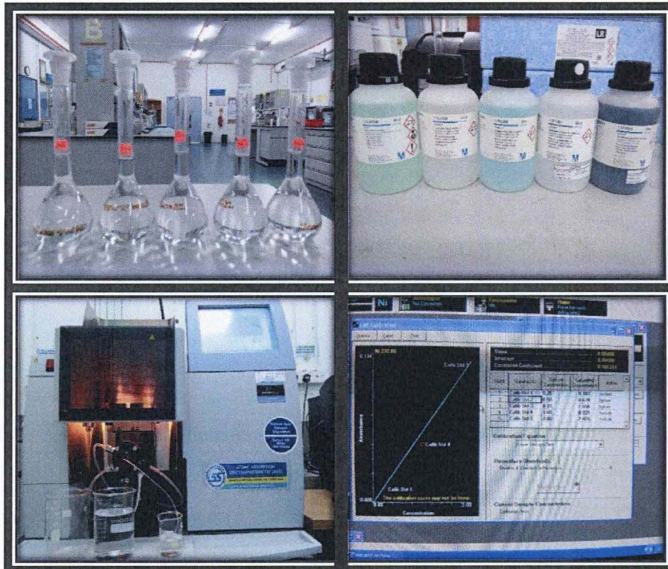
Figure 3.15 Heavy Metals Test by Using Method of AAS
