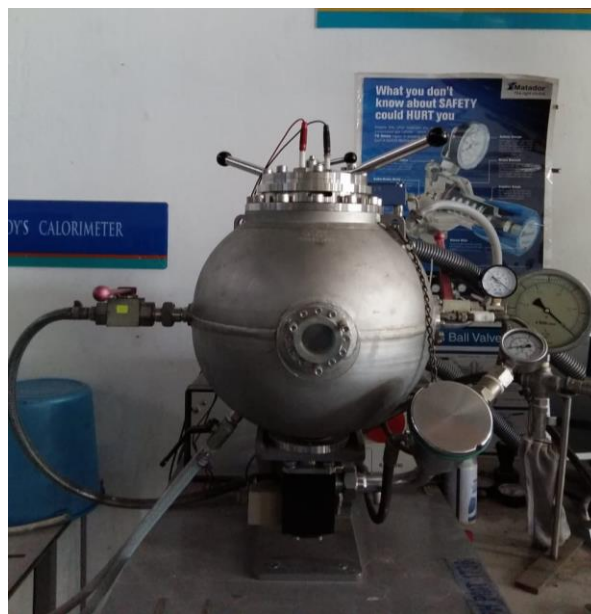
Figure 1. The standard 20 L spherical vessel
