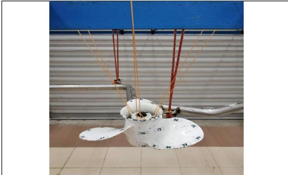
**Figure 4.** Hanging propeller structure under free-free boundary condition.
