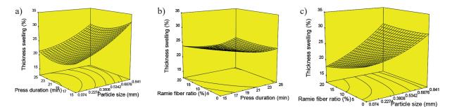
**Figure 2.** Response surface 3D plots on thickness swelling of hybrid bio panels (a) particle size and press durations, (b) ramie fiber ratio and press durations, and (c) ramie fiber ratio and particle size
