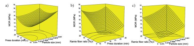
**Figure 3.** Response surface 3D plots on MOR of hybrid bio panels (a) particle size and press durations, (b) ramie fiber ratio and press durations, and (c) ramie fiber ratio and particle size
