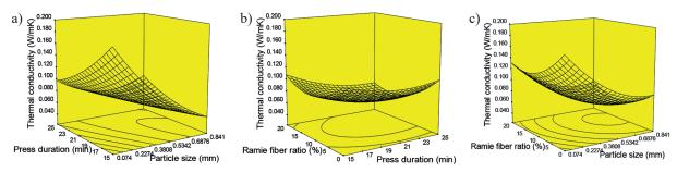
Figure 4. Response surface 3D plots on thermal conductivity of hybrid bio panels (a) particle size and press durations, (b) ramie fiber ratio and press durations, and (c) ramie fiber ratio and particle size
