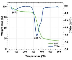
Figure 5. TGA and DTGA curve of hybrid bio-panels based on OPT
