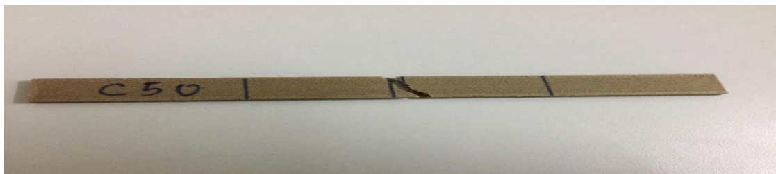
Figure 4(b). 50% infill percentage Coconut Wood with Concentric infill pattern.
