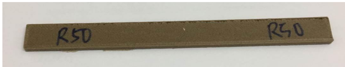
Figure 3(c). 50% infill percentage Coconut Wood with Rectilinear infill pattern.
