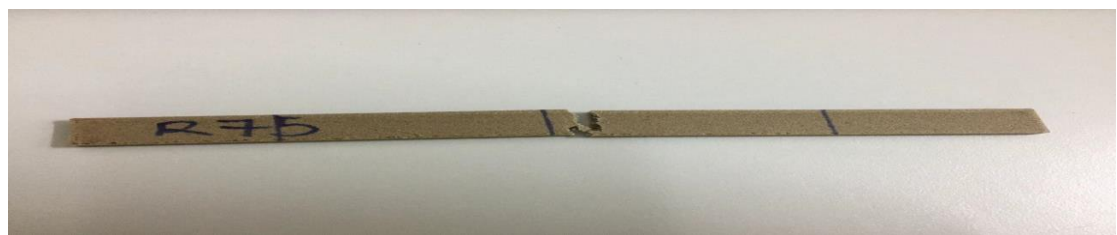
Figure 4(c). 75% infill percentage Coconut Wood with Rectilinear infill pattern.
