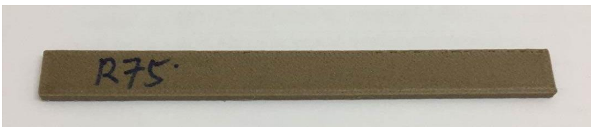
Figure 3(d). 75% infill percentage Coconut Wood with Rectilinear infill.
