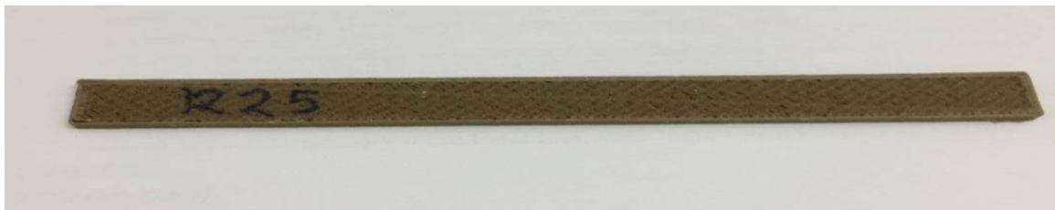
Figure 3(b). 25% infill percentage Coconut Wood with Rectilinear infill pattern.
