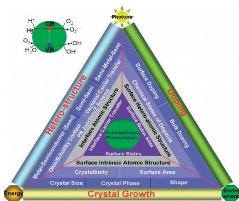
Figure 1.1: Correlation of key factors in crystal growth, doping and heterostructuring of semiconductors for photocatalysis. (CB: conduction band; VB: valence band)
