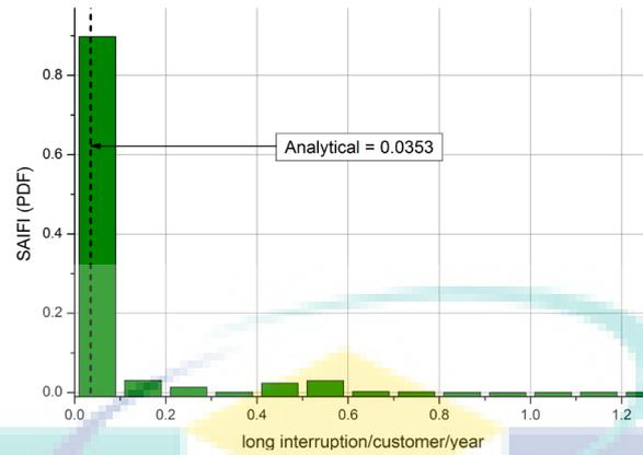
Figure 19: SAIFI (PDF) for LV Network with protection devices
