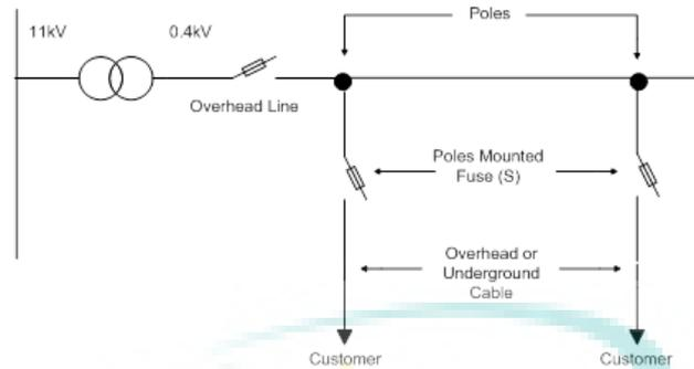
Figure 10. Typical Arrangement for LV overhead distribution systems [37]
