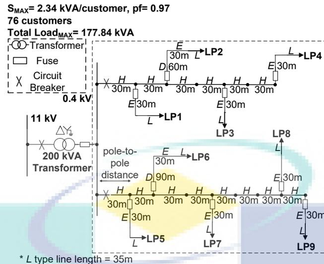
Figure 12: LV SU distribution network with fuse protection [37]–[43]
