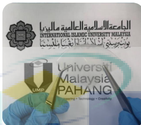
Figure 4.1 A transparent thin film of CMC-PVA of the BPe system
