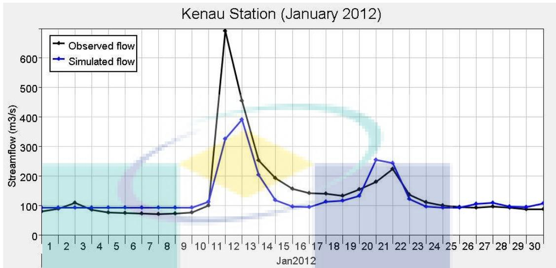
Figure 4.4 The validated hydrograph for two scenarios; a) Moderate flow scenario in February 2011 b) High flow scenario in January 2012
