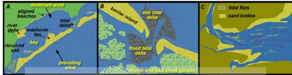
Figure 2.5 Estuary models a) Microtidal b) mesotidal c) macrotidal
