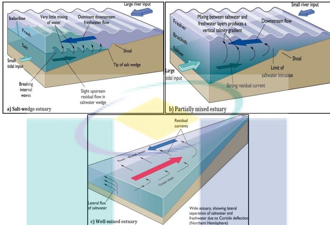
Figure 2.1 The mixing classification in estuary a) Salt-wedge estuary b) Partially mixed estuary c) Well-mixed estuary
