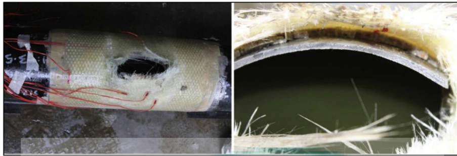
Fig. 12. Failure pattern of the repaired pipe.
