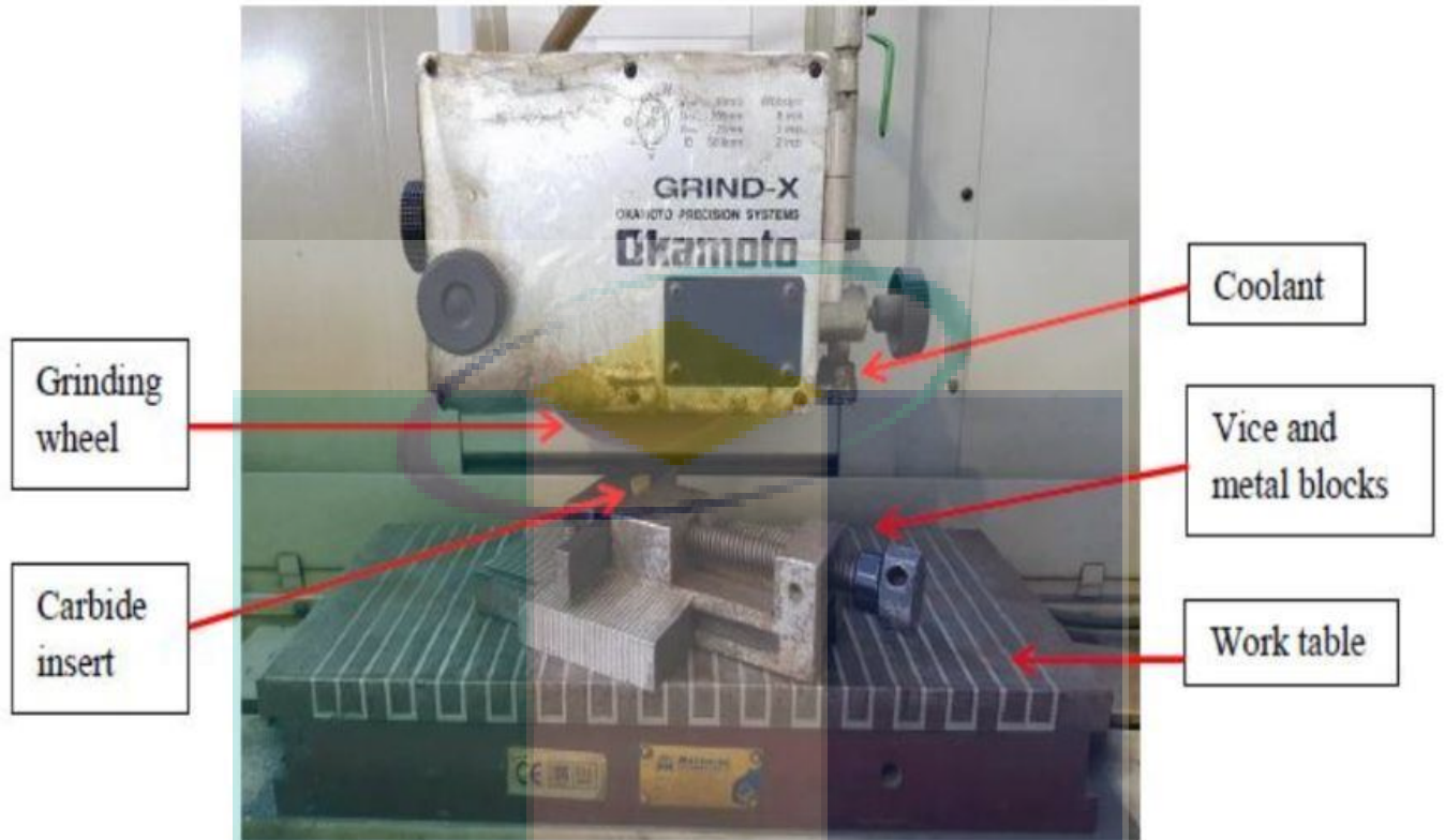
Surface texturing by grinding process
