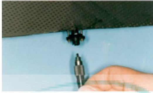
Figure 2.29 Embedded connector inside the composite together with optical fibre Source: Ramakrishnan et al. (2016).
