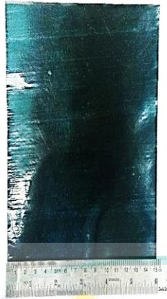
Figure 3.15 Prepreg unidirectional fibre of CFRP
