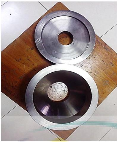
Figure 3.22 Material clamper
