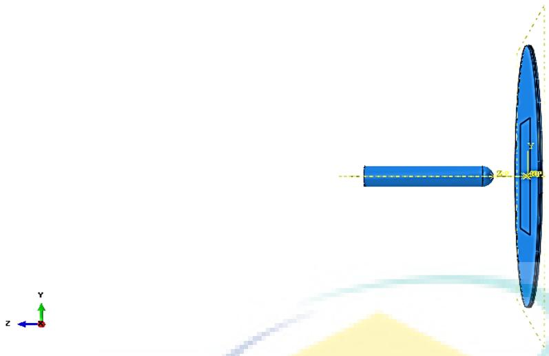
Figure 3.7 Indenter and FML in Assembly
