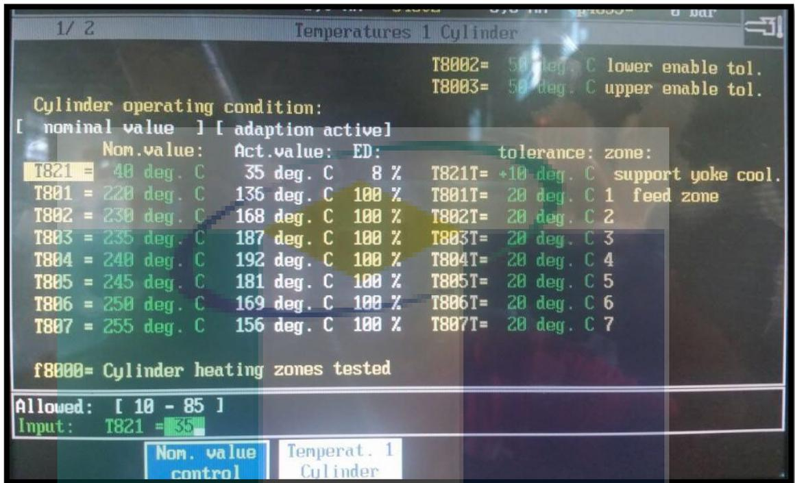
Figure 3-7 Temperature variance for injection process
