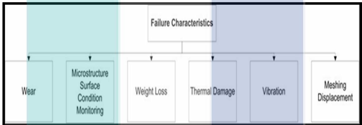
Figure 2-1 Types of failure characteristics for polymer gear
