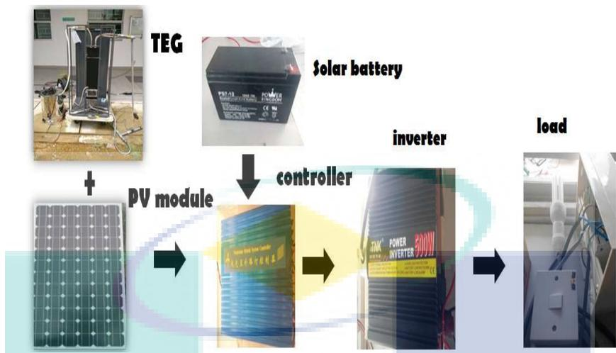
Figure 3.16: Hybrid PV-TEG hardware development
