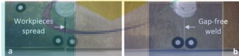
Fig. 2.1. Gap between specimens at the start of the FSW process based on the condition of clamping [19]. (a) without lateral pressure, (b) with lateral pressure.
