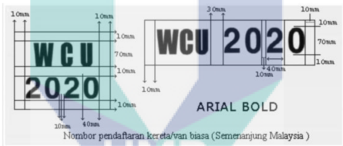
Figure 2.1: Standard plate size from JPJ [4]
