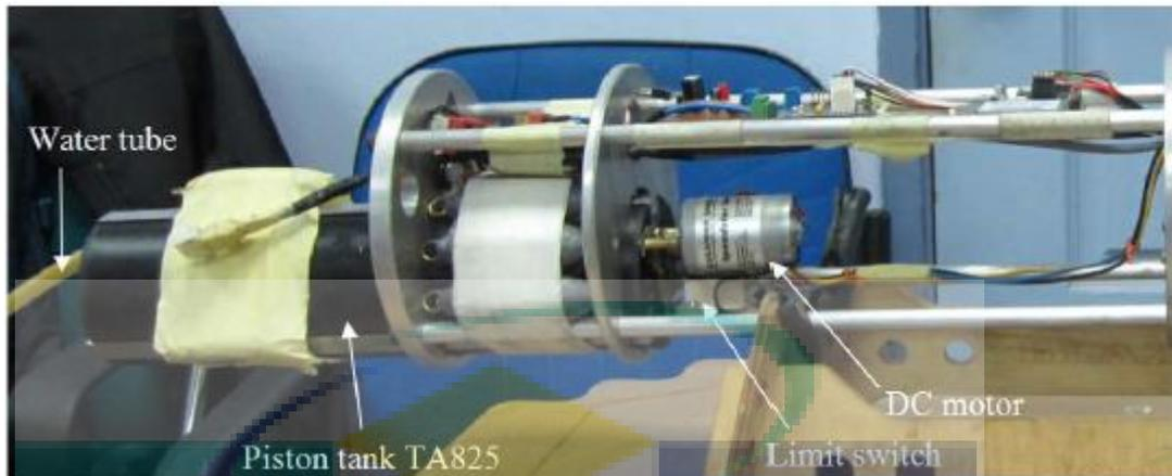
Figure 3-6 Ballast tank installation and configuration
