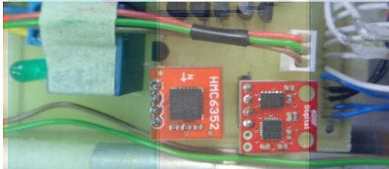
Figure 3-12 IMU and compass
