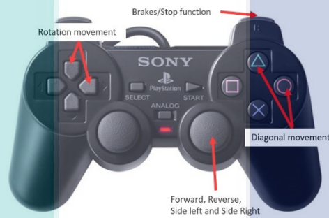
Fig. 15. Key-Binding control of Joystick used for MHeLFAGV remote controller.
