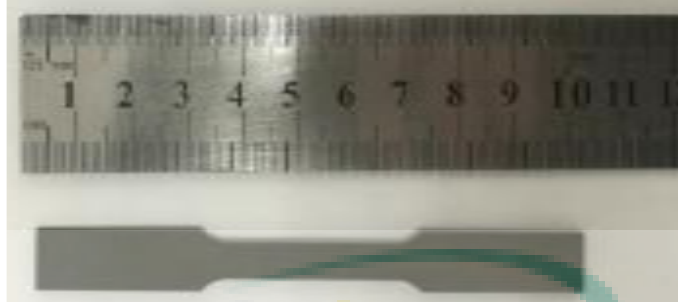
Figure Error! No text of specified style in document..58 Specimen for tensile strength test
