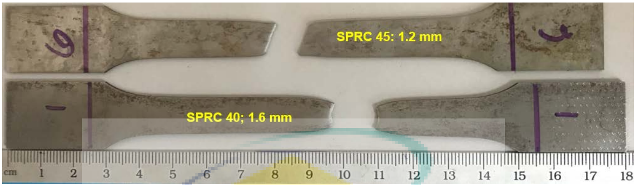
Fractured sample of base metal SPRC 40 and SPRC 45
