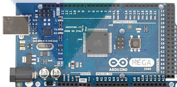
Figure 3-4 Arduino Mega 2560 that is used as the microcontroller to carry out visual analyzing and system design algorithm
