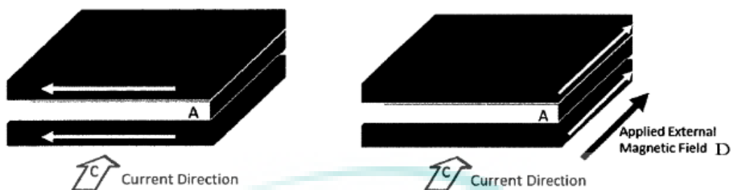
Figure 2: A diagram illustrating of GMR. a) GMR film layers without an applied magnetic field showing directions of magnetic moments b) GMR layers in the presence of an applied magnetic field
