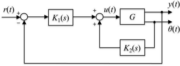
Fig. 1: PID control system for liquid slosh problem
