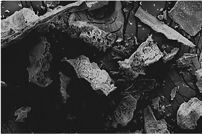
Fig. 4. SEM micrograph of RHA particles at a magnification of 1000X.
