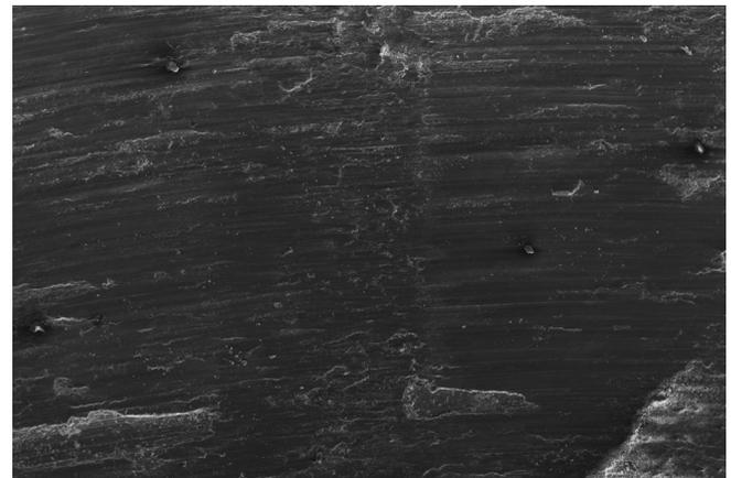
Fig. 7. SEM micrograph of FSPed AA6061/6 vol% RHA.
