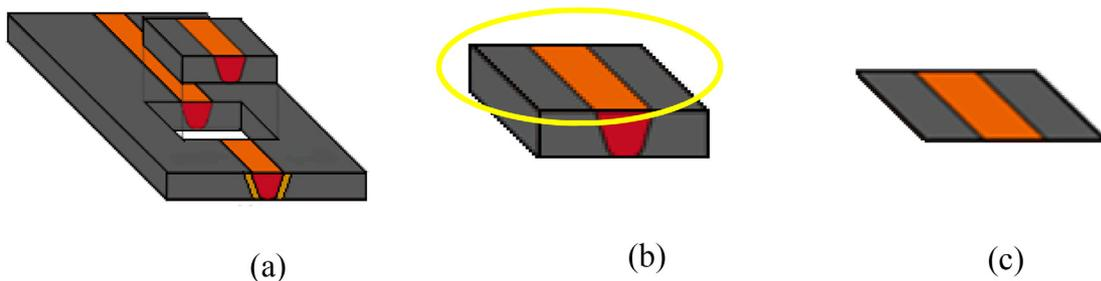
Fig. 1. (a) Specimen was cut perpendicular to traversed path using EDM wire cut, (b) specimen for wear test and (c) area for morphology observation.
