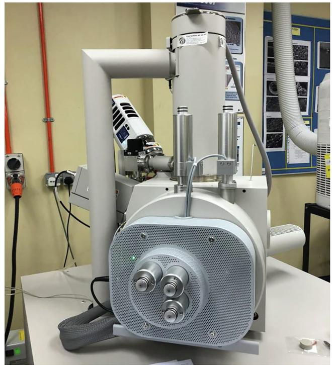
Fig. 3. SEM equipped with EDX.
