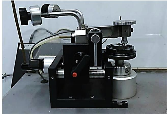
Fig. 2. Pin-on-disc tribometer.
