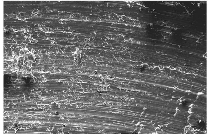
Fig. 6. SEM micrograph of FSPed AA6061.
