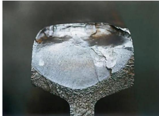
Figure 6. Internal defect of the head in the weld. [31]
