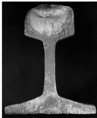
Figure 5. Rail kidney defect. [31]
