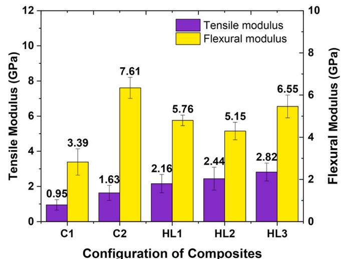
Fig. 5. Tensile and flexural modulus of hybrid laminated composite.
