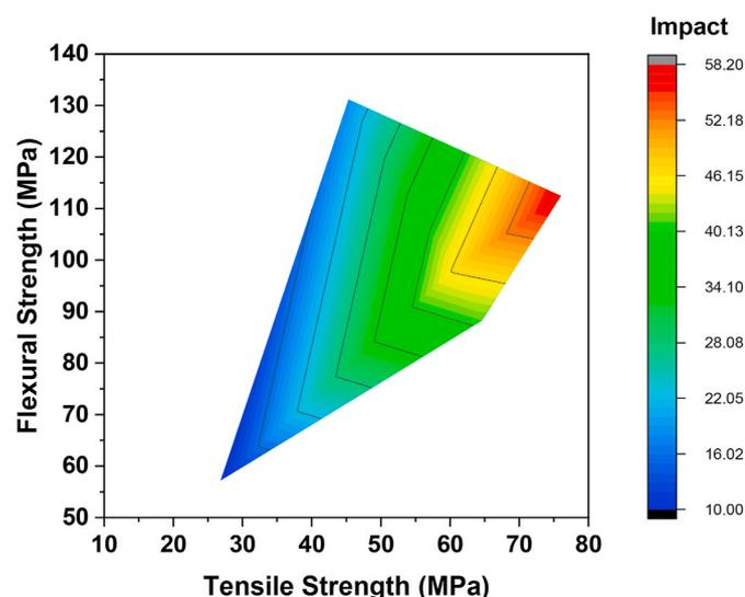
Fig. 6. Relationship impact strengths, tensile and flexural strength of hybrid laminated composites.
