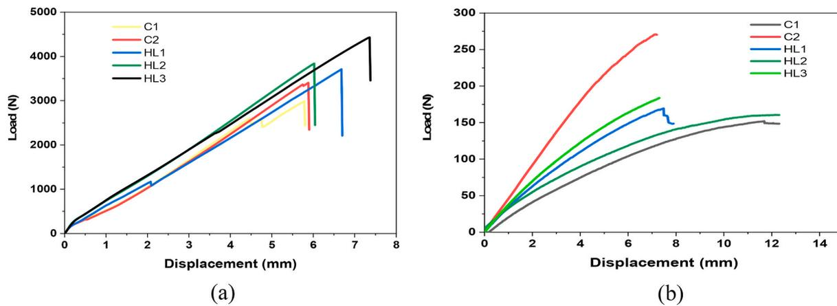
Fig. 3. Load vs displacement of hybrid laminated composite (a) Tensile test and (b) Flexural test.
