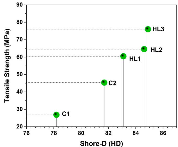
Fig. 7. Correspondence hardness and tensile strength of hybrid laminated composites.
