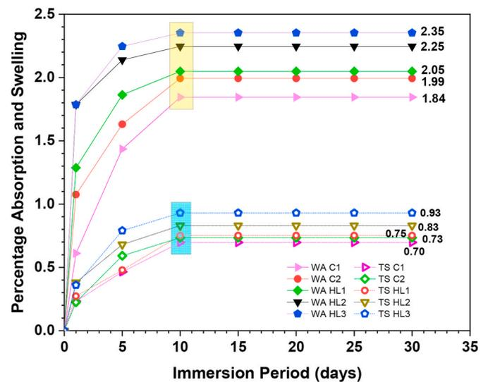
Fig. 2. WS and TS of hybrid laminated composites with different type.
