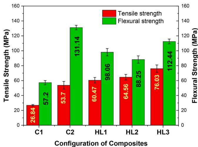
Fig. 4. Tensile and flexural strength of hybrid laminated composite laminates.
