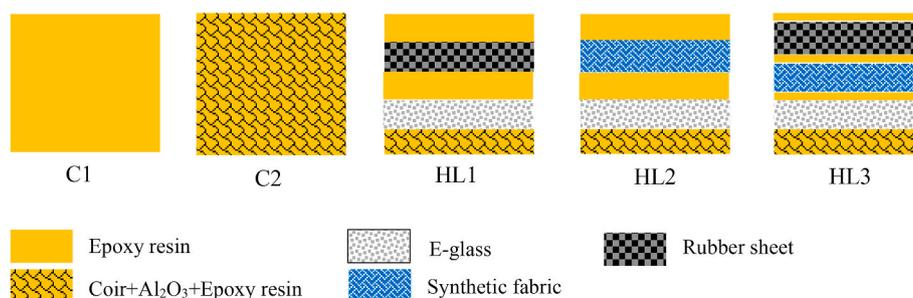
**Fig. 1.** Illustration of hybrid laminated composites configuration.
