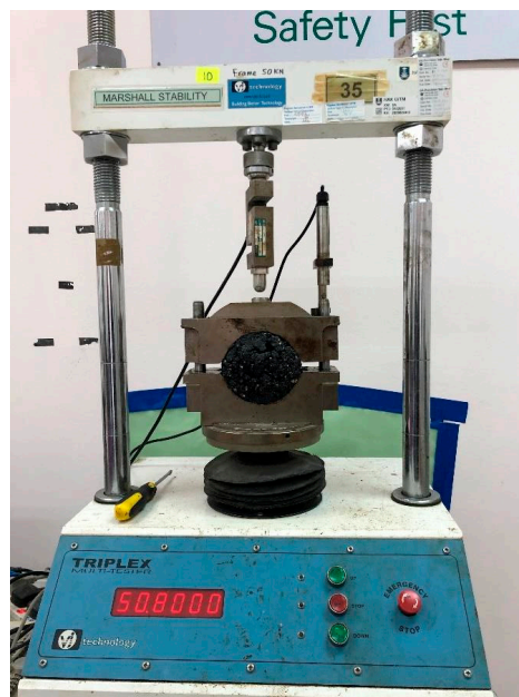
Figure 3. Marshall stability test.
