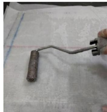
Fig. (4). Rolled the wet GFRP sheet to removed excess epoxy resin and trapped air bubbles.
