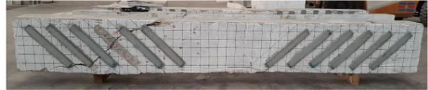
Fig. (21). The strengthened beam using GFRP.
