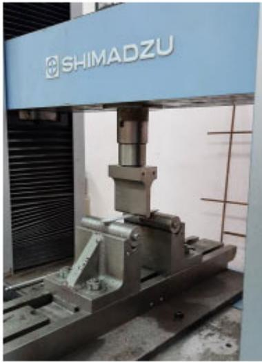
Fig. (12). Flexural test conducted on the GFRP strips.
