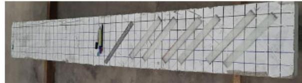
Fig. (8a). The location of each GFRP strip was sketched.
