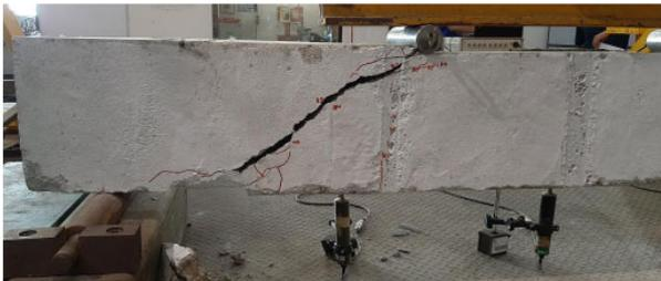
Fig. (19). Crack pattern of the control beam.
