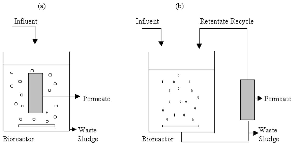
**Figure 2.3:** (a) Internal Membrane Bioreactor and (b) External Membrane Bioreactor Reactor (Recirculated)
