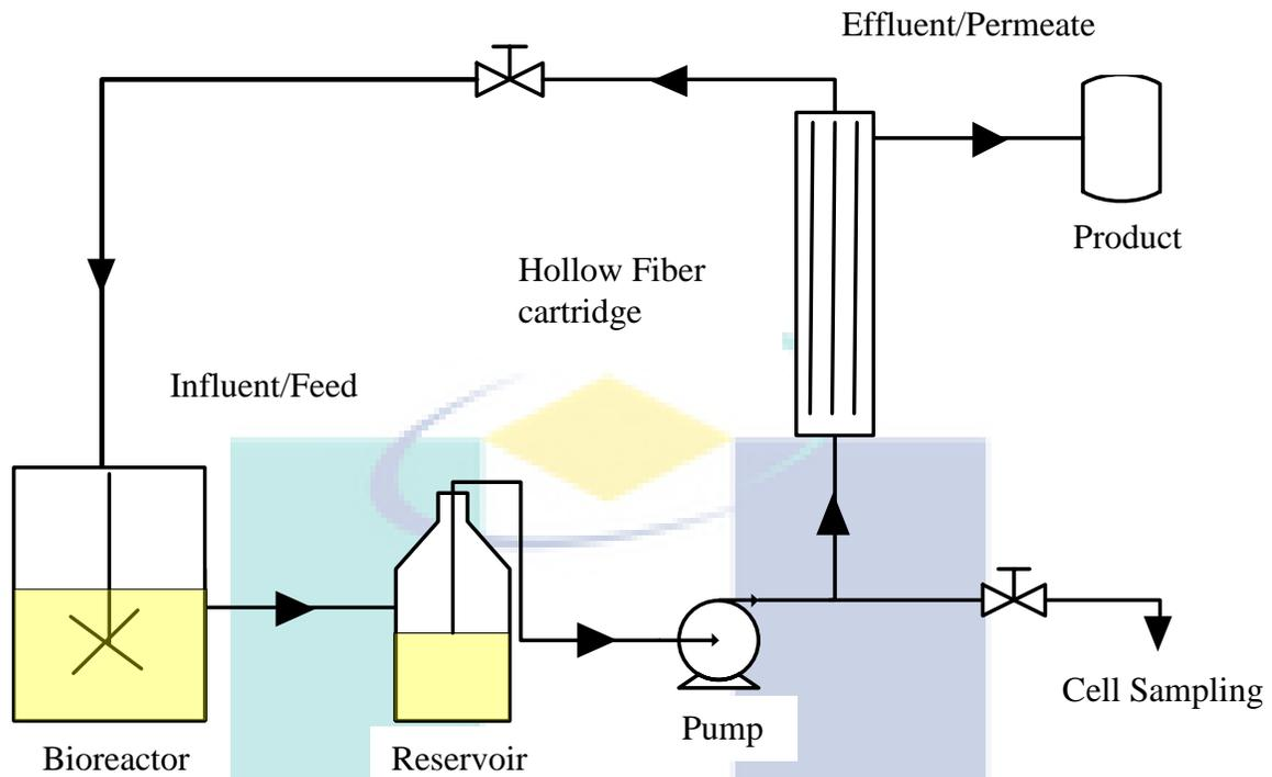
**Figure 3.6:** Diagram of Membrane Bioreactor (MBR)
