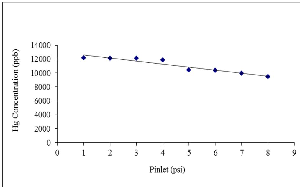
**Figure 4.22:** Mercury (14000 ppb) removal using membrane microfiltration system
