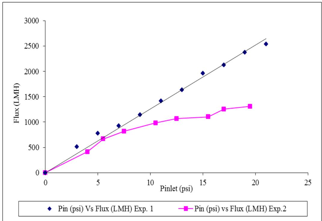
**Figure 4.21:** Permeate flux for de-ionized water (Exp. 1) and Hg solution at 14000 ppb (Exp. 2) with respect to inlet pressure,  $P_{inlet}$ .
