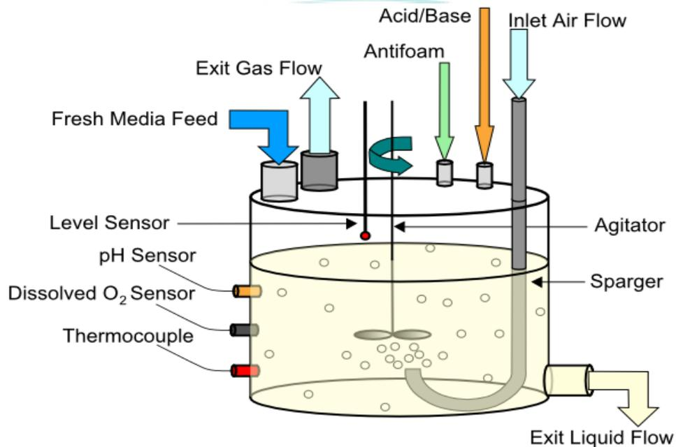
**Figure 2.8:** Diagram of bioreactor for *P. putida* cultivation
