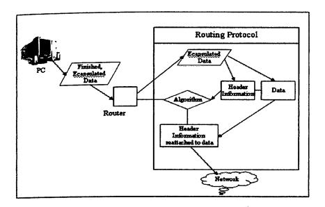
Figure 2.2: The Process Used By Routing Protocol (J.F.DiMarzio, 2002).
