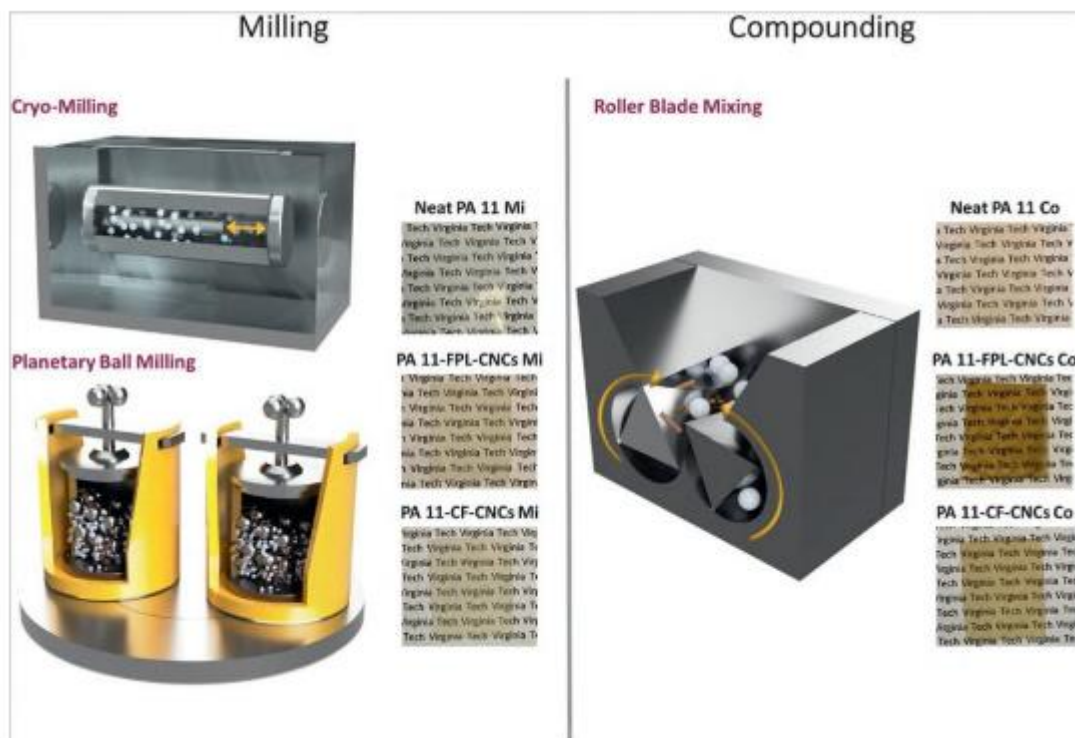
Fig. 13.2 PA11 and PA11/CNC nanocomposite film fabricated via melt compounding with preprocess with milling (left) and without milling (right).
