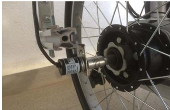
Figure 5. The position of rotary encoder installed on EPW.
