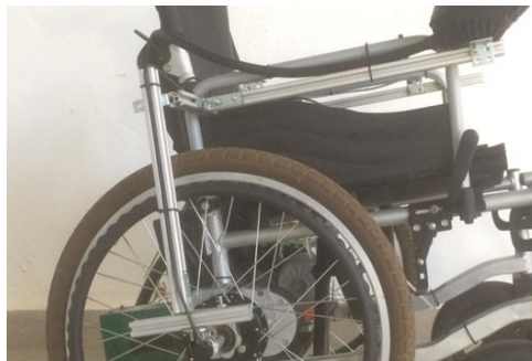
Figure 3. The additional frame attached to the frame of the EPW for the sensor installation purposes.
