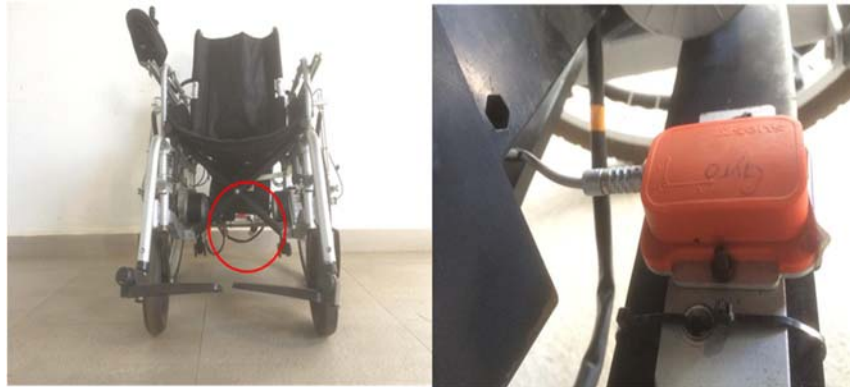
Figure 6. The position of gyroscope sensor being installed on EPW.
