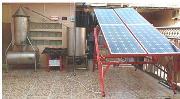
Figure 1. Photovoltaic circuit without distillation.
