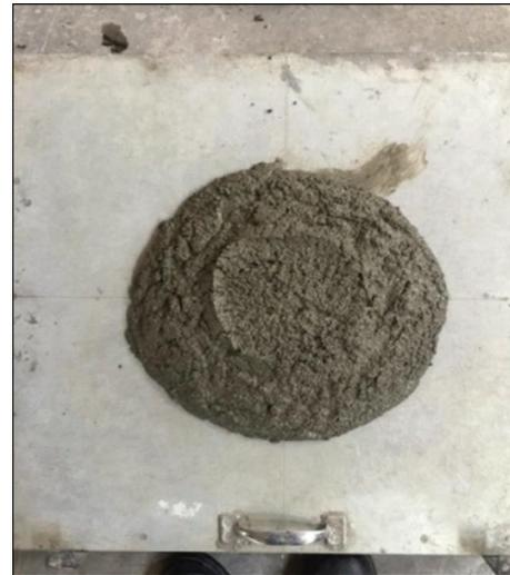
FIGURE 3: Flow table test.
