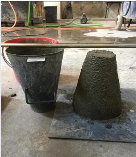
FIGURE 2: Slump test.
