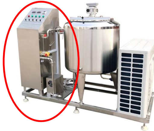
Figure 3. Electric control panel of pasteurizer
