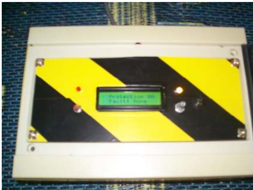
Figure A1: Auto Re-closer ELCB with casing
