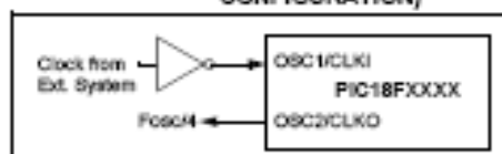
FIGURE 2-4: EXTERNAL CLOCK INPUT OPERATION (EC AND ECPLL CONFIGURATION)
