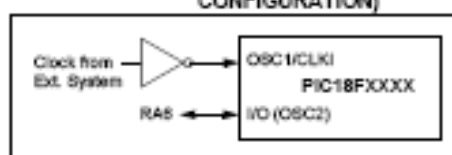
FIGURE 2-5: EXTERNAL CLOCK INPUT OPERATION (ECIO AND ECPIO CONFIGURATION)
