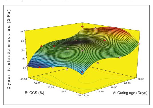
Fig. (7). Response surface plot indicating the effects of curing age and crushed cockle shells content on the dynamic elastic modulus of mortar.
