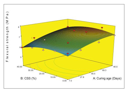
Fig. (6). Response surface plot indicating the effects of curing age and crushed cockle shell content on flexural strength of mortar.
