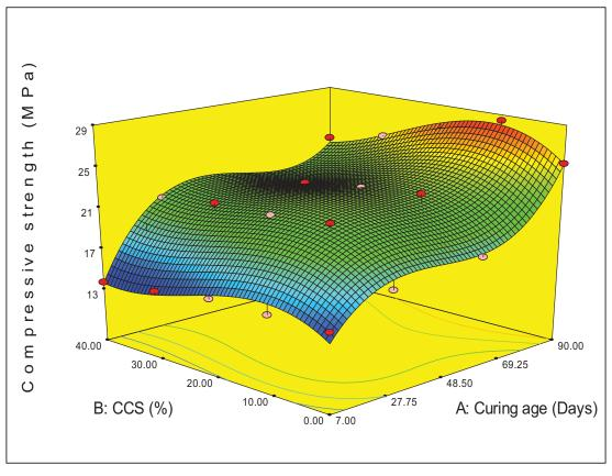
Fig. (5). Response surface plot indicating the effects of curing age and crushed cockle shell content on compressive strength of mortar.
