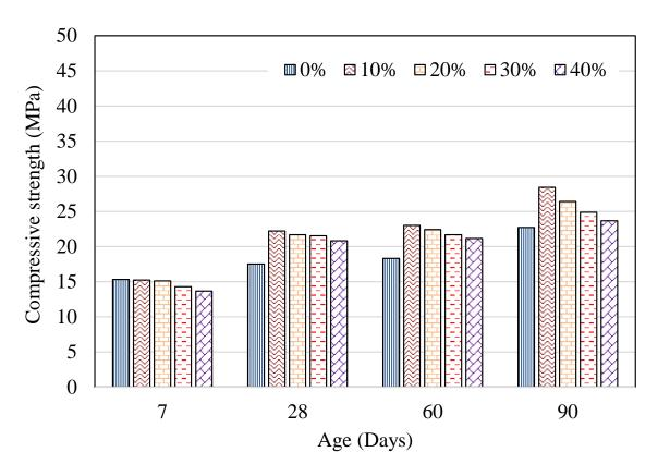
Fig. (2). Compressive strength of CCS mortars.
