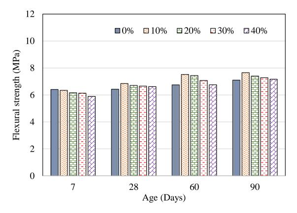
Fig. (3). Flexural strength of CCS mortars.
